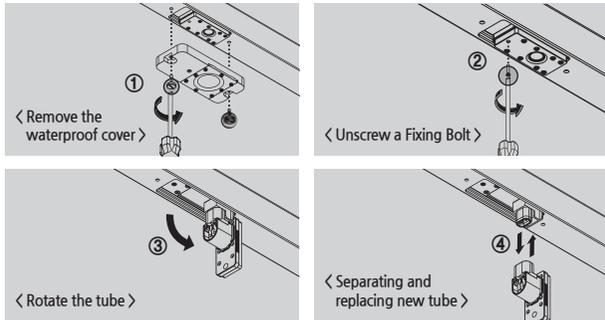
\* Please implement the tube reset in a controller after replacing a tube. (Refer to SXC-10BT/BL manual)
