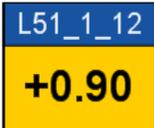
The ID and the current measured value appear in the sensor icon. According to the setting, the grayed-out graph of the measured values is displayed on the background for 6 seconds.
