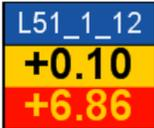
If the measured value of the electrostatic voltage exceeds the set range, the most recent exceeding value blinkers and appears at the bottom.
