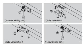
\* Please implement the tube reset in a controller after replacing a tube. (Refer to SXC-10BT/BL manual)
