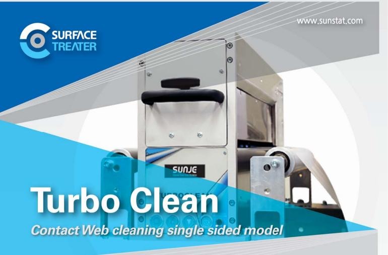
The cleaning takes place thanks to a roller coated with special rubber which by rotating picks up from the surface of the film all dirt particles and then the particles are deposited on an adhesive roller.
