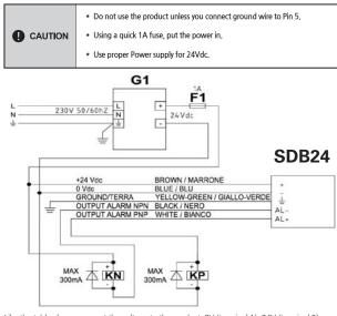
Like the table above, connect the voltage to the product. 0V (terminal 1), 24V (terminal 2), ground (terminal 4). To connect 24Vdc power supply to the product, you should connect ground wire. (Pin 4 from female connector)
