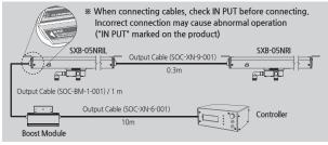
\* SXB-05NRIL cannot be used alone and can only be used when SXB-05NRI is connected. The use of the Boost Module is mandatory.
