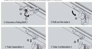
\*\* After replacing the Tube, run "Tube Reset" on the controller. If the reset process is not performed, the replaced tube will not work.
