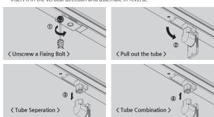
\*\* After replacing the Tube, run "Tube Reset" on the controller. If the reset process is not performed, the replaced tube will not work,
