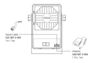
Connect the Signal Cable (SUC-MT-2-005) when you want to control the SBL-80S from the outside or check its operational status.
