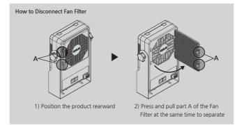
\* You can assemble the Fan Filter coupling in the reverse order of the separation method.
