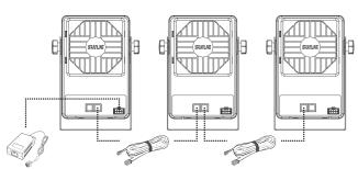
Adapter (1,5m) Output: DC 24V, 2,5A Extension Cable (1m)\_OptionExtension Cable (1m)\_Option
