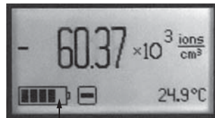
Battery Level : Each missing bar represents a drop of approximately 20% of battery's capacity.
